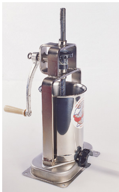
(a) A small sausage stuffer fitted with a medium nozzle. This stuffer holds 5 lb (2.3 kg) meat at a time.
