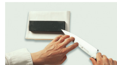
(a) Hold the knife firmly. Start with the tip of the knife against the stone as shown, and hold the edge against the stone at a 20-degree angle. Use the guiding hand to keep an even pressure on the blade.
