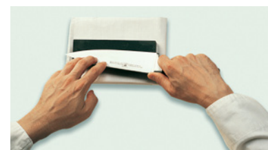
(d) Draw the knife across the stone all the way to the heel of the blade.
