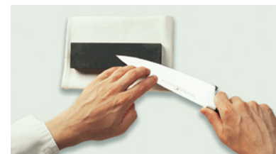
(b) Start to draw the knife over the stone. Press very gently on the blade.
