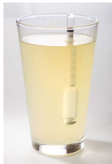
Testing a sorbet mix with a hydrometer.
